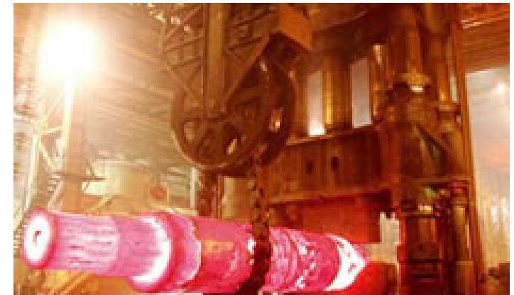
Processing of half-speed turbine rotor of 1100MW nuclear power
