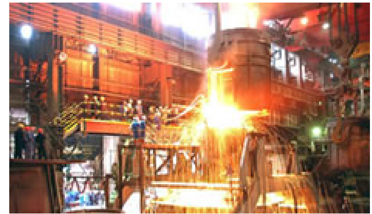
Vacuum casting of 560 ton ingot
